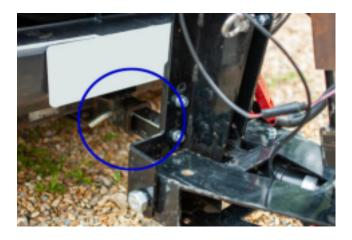
Connect the electrical connectors from the plough to the corresponding connectors on the vehicle.
