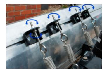
Caster wheel adjustment, the castor wheels can be raised and lowered by twisting the top adjuster to aid with fitting and removal of the plough from the vehicle.
