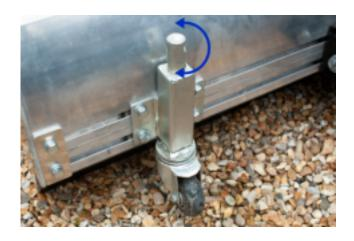
Spigot height adjustment, the 50mm spigot can be bolted to the headstock in numerous positions. This helps to keep the plough at the correct height off the ground depending on chassis height and blade wear. This can best be done with the plough removed from the vehicle. Remove the four securing bolts from the spigot and replace them in the holes that best line up when the spigot is set at the correct height to the headstock.
